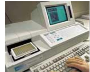
Read OD results (450 nm filter), 2-20 min after stop
